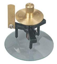
It carries a circular scale divided into 100 equal parts. (In some cases it is divided into 50 equal parts). The edge of the circular scale is very close to the metal strip and the metal strip is used also as a reference line for taking the circular scale reading. The disc & scales are brass lacquered & legs are made of steel black painted.
